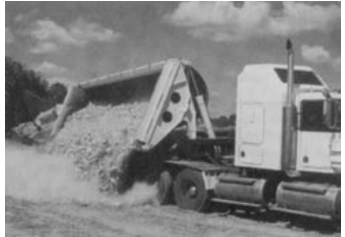
Photo 7: Flexible Side Tipper from 6mm Bisplate 360
