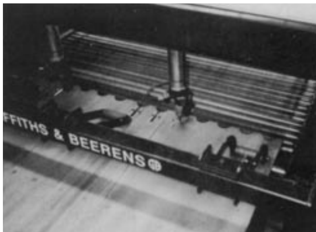
Photo 6 — Chain Saw Guide Bars Laser Cut from Bisplate 500
