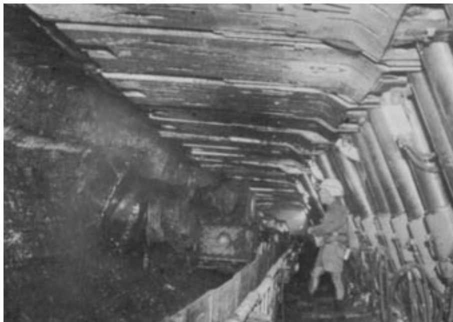
Photo 9: Underground Longwall Mining Operation – using roof supports constructed from Q&T structural grades and pan lines using Q&T wear plates.
