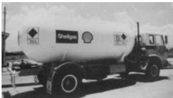
Photo 3: Transportable Road Tanker Manufactured to AS 1210 from AS 3597 grade 700PV
