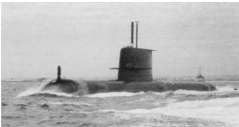
Photo 1: HMAS Collins Class Submarine, from locally manufactured Q&T material, undergoing sea trials.
