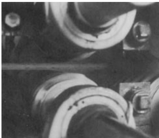
Photo 5: Roller Quenching of Q&T Steels at Bisalloy Steels
