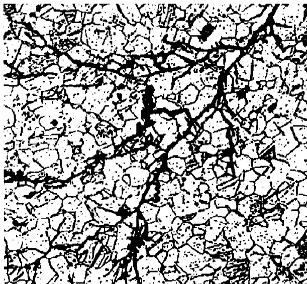
Fig. 6: Stress Corrosion Cracking in a Grade 304 Stainless Steel Hot Water Vessel
