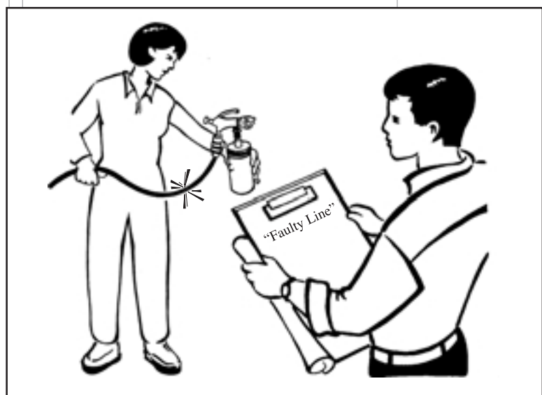
Figure 4 – Identifying plant hazards – inspection of empty spray apparatus shows there is a hole in the supply line
